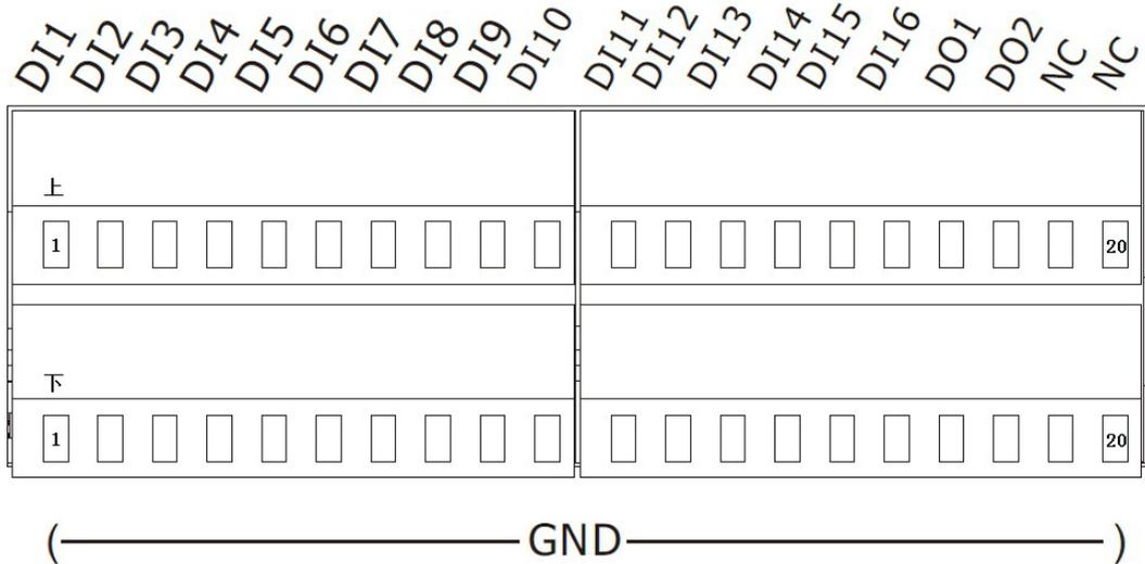
Fig. 3-2-220Pin Socket Interface
